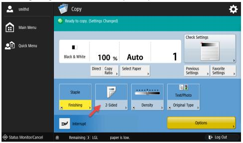
2. Select the desired option from the available choices. For example, to copy a single-sided original to a double-sided copy, press the **1-Sided > 2-Sided** button on the touch panel **(1)**. Then press the **OK** button **(2)**.
