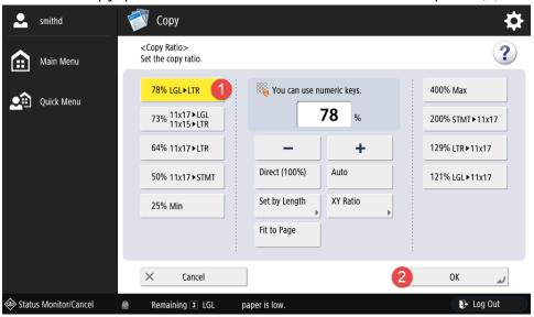
3. The **Copy Ratio** button will be highlighted, and you selected enlargement / reduction settings will be displayed on the top of the settings screen.
